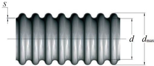
Figure 1 Profile of transverse corrugated pipe made of stainless steel AISI 304 [26]
