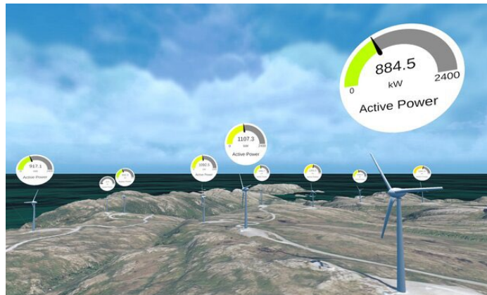
Figure 9. Descriptive digital twin with text and gauges showing active power of each turbine [5] (under CC BY 4.0).
