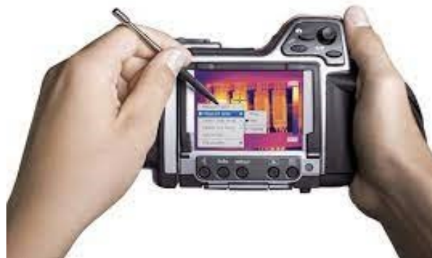
Figure 3 Equipment for measuring the temperature of landfill gas - thermal imaging camera FLIP T335
