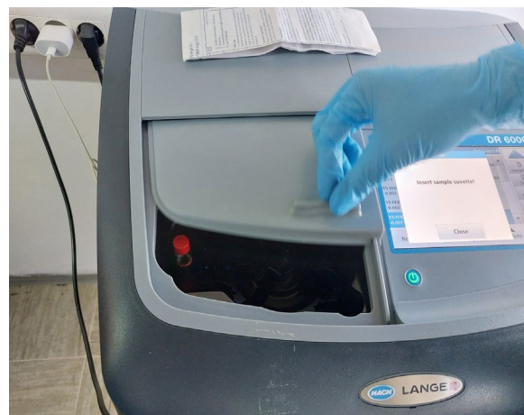
Figure 22. Closing the lid, so the spectrophotometer can start measurement
