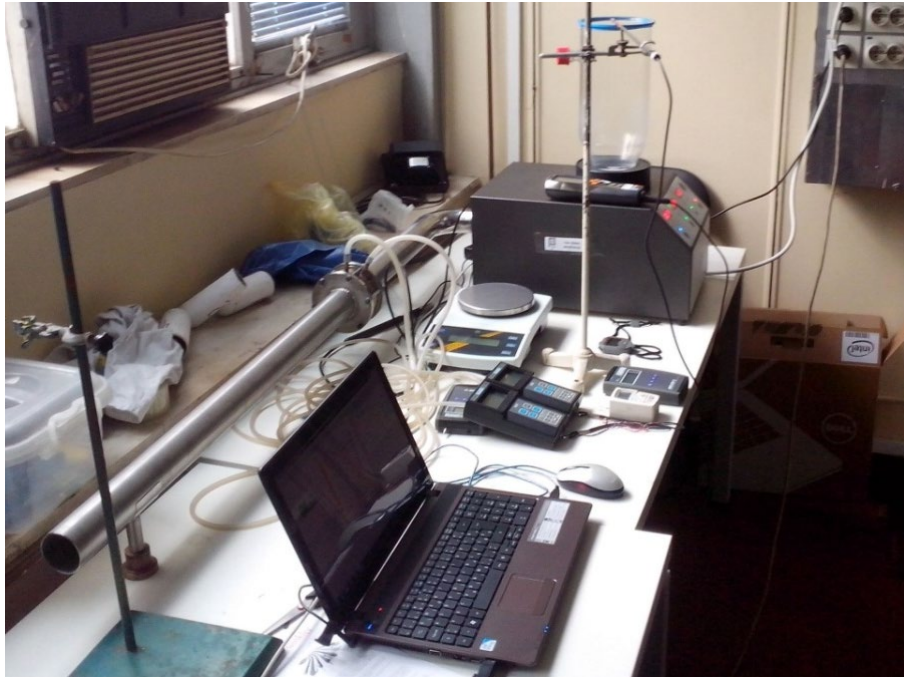
Figure 2. Dryer Sherwood Tornado M501 with built-in orifice plate [1]
