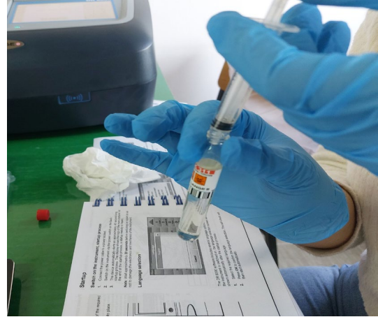
Figure 18. Putting the specific amount of sample into the LCK cuvette
